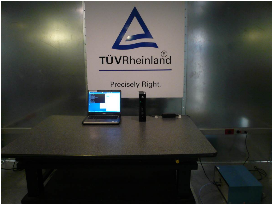
Figure 13: AC Conducted Emission Test Setup (Front View)
