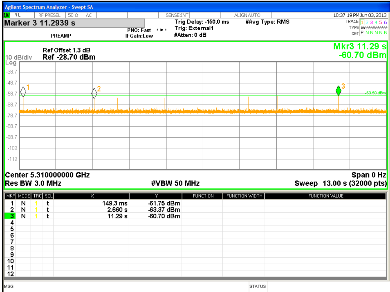
Figure 9: Long Pulse Radar Type at 5310 MHz (11-20µs Pulse Width, 200-500µs PRI, 8-20 Bursts)
