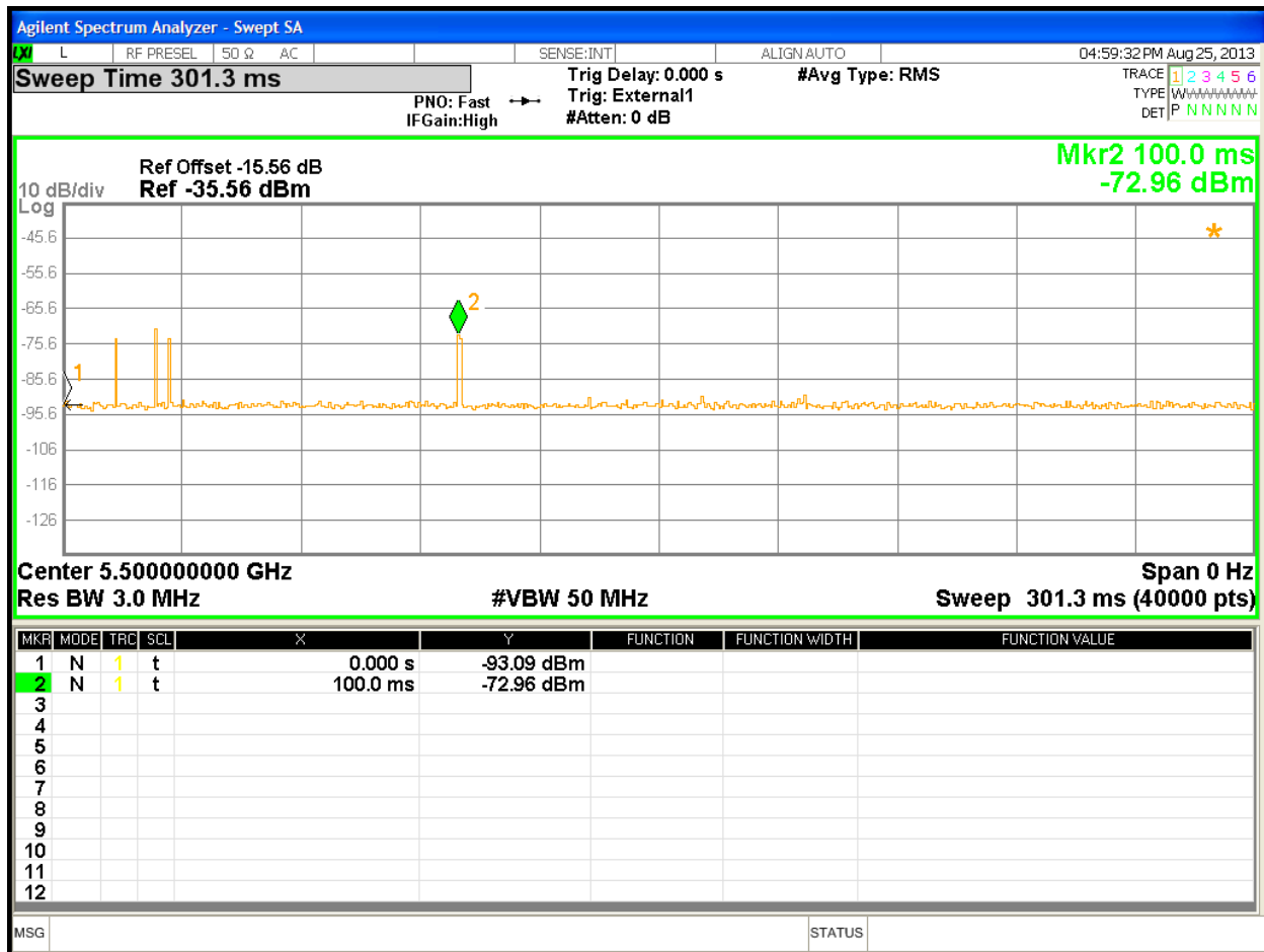
Figure 21: Channel Move Time and Channel Closing Transmission Time using Short Pulse Radar Waveform 1 1 in Master Mode for 20 MHz Bandwidth - (Close-up)
