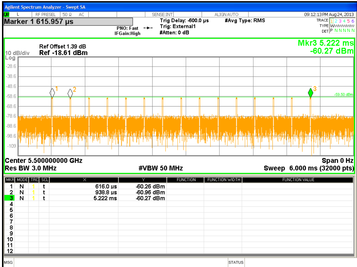
Figure 8: Short Pulse Radar Type 4 at 5500 MHz (50-100 \mu S Pulse Width, 1000-2000 \mu S PRI, 12-16 Pulses)
