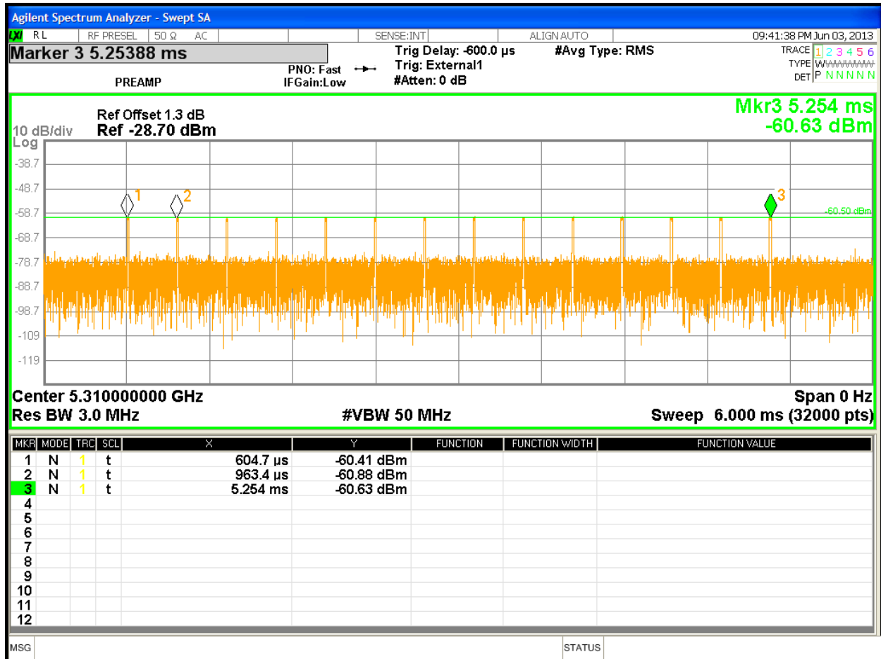
Figure 7: Short Pulse Radar Type 4 at 5310 MHz (50-100μS Pulse Width, 1000-2000μS PRI, 12-16 Pulses)
