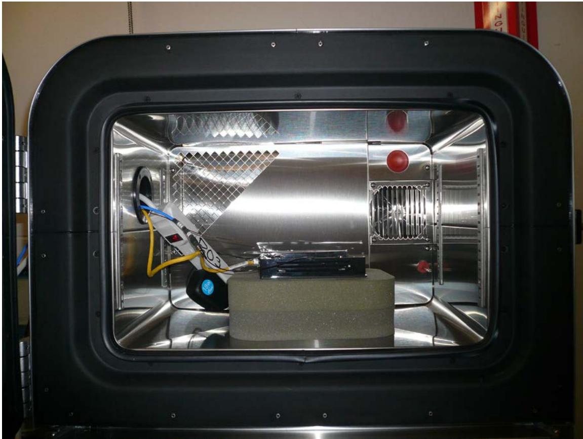
Figure 11: Extreme Condition Test Setup – Inside Thermo Chamber
