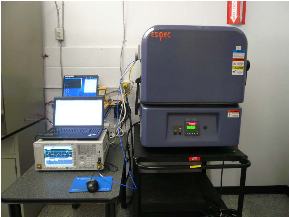
Figure 12: Extreme Condition Test Setup – Outside Thermo Chamber
