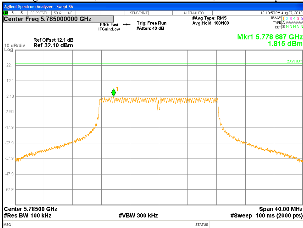
Figure 192: PPSD, 5785 MHz at 802.11n 802.11A, Chain 3 – 6 Mbps
