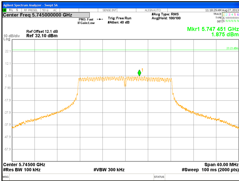
Figure 185: PPSD, 5745 MHz at 802.11n 802.11A, Chain 0 – 6 Mbps
