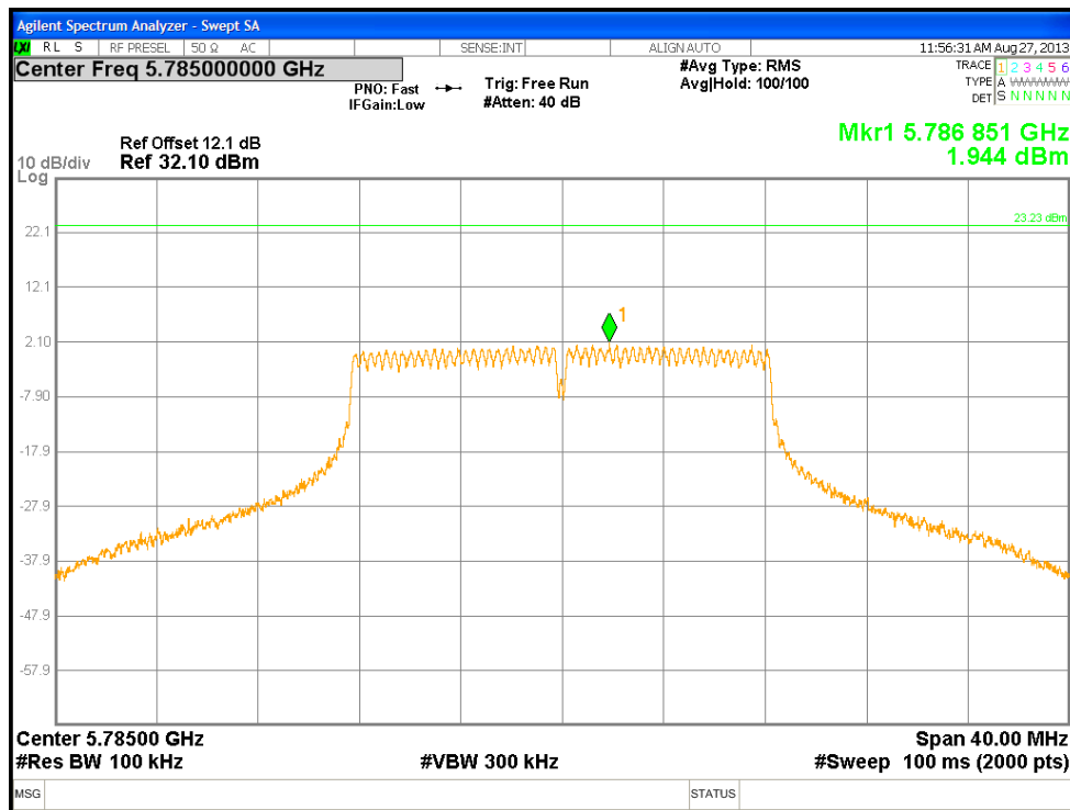
Figure 189: PPSD, 5785 MHz at 802.11n 802.11A, Chain 0 – 6 Mbps
