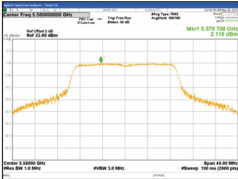
Figure 78: Power Spectral Density, 5580 MHz at 802.11n, Chain 0 – 6.5Mbps
