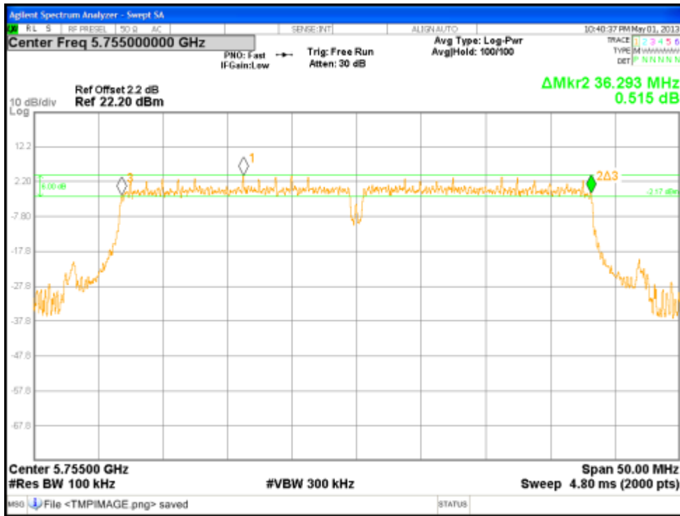
Figure 51: DTS Bandwidth at 5755 MHz, Chain 3
