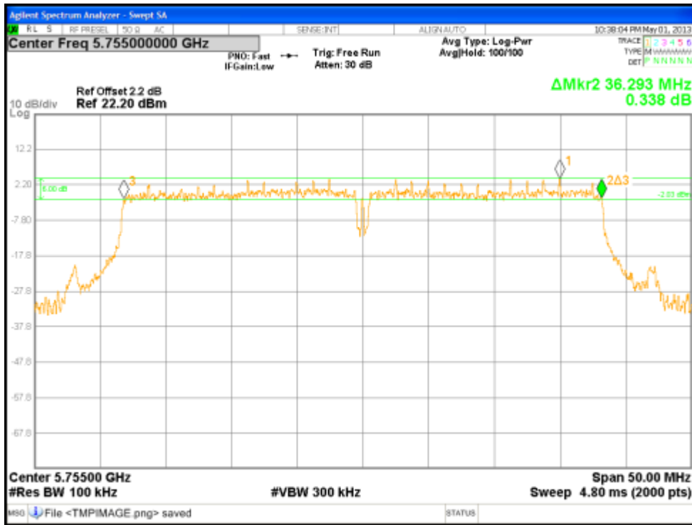
Figure 47: DTS Bandwidth at 5755 MHz, Chain 1
