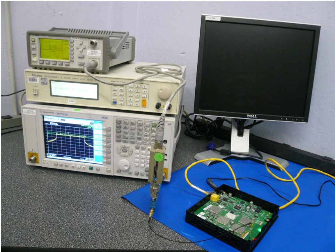
Figure 10: RF Conducted Test Setup - Closeup
