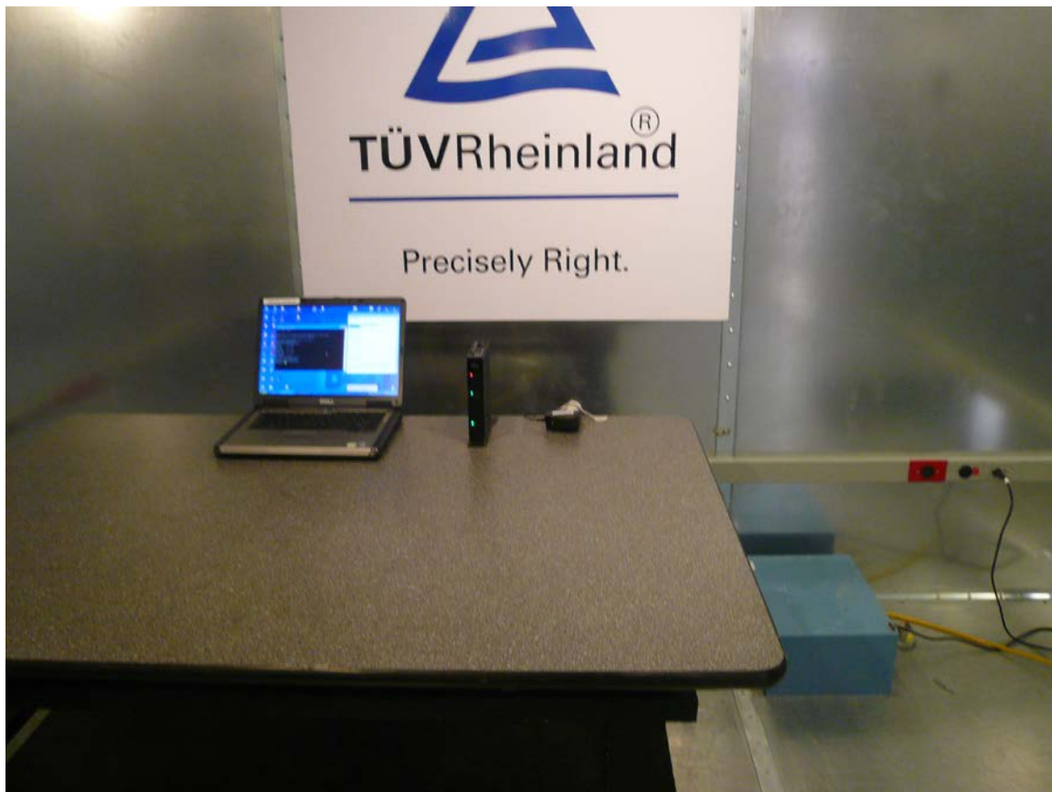
Figure 14: AC Conducted Emission Test Setup (Front View)
