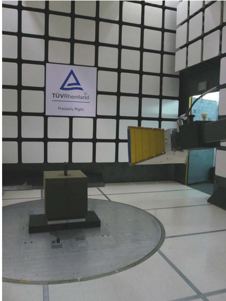
Figure 4: Test Setup for 1GHz to 18GHz (Rear View) – Y-Axis
