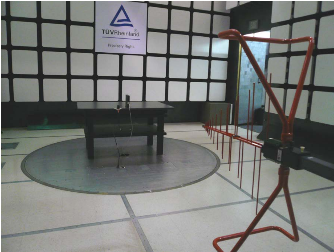
Figure 2: Test Setup for 30 MHz to 1000MHz (Rear View) – Y-Axis
