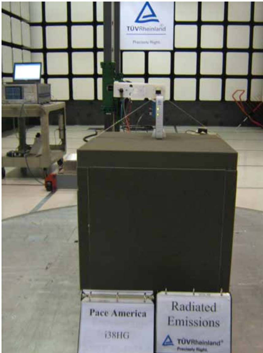
Figure 5: Test Setup for 18 GHz to 26GHz (Front View) – i38HG on Vertical Position
