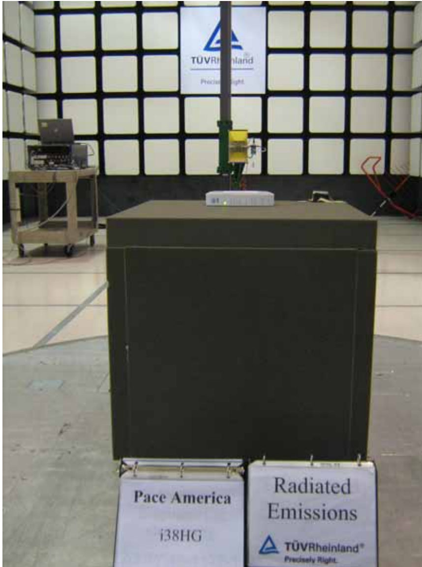
Figure 3: Test Setup for 1GHz to 18GHz (Front View) – i38HG on Horizontal Position
