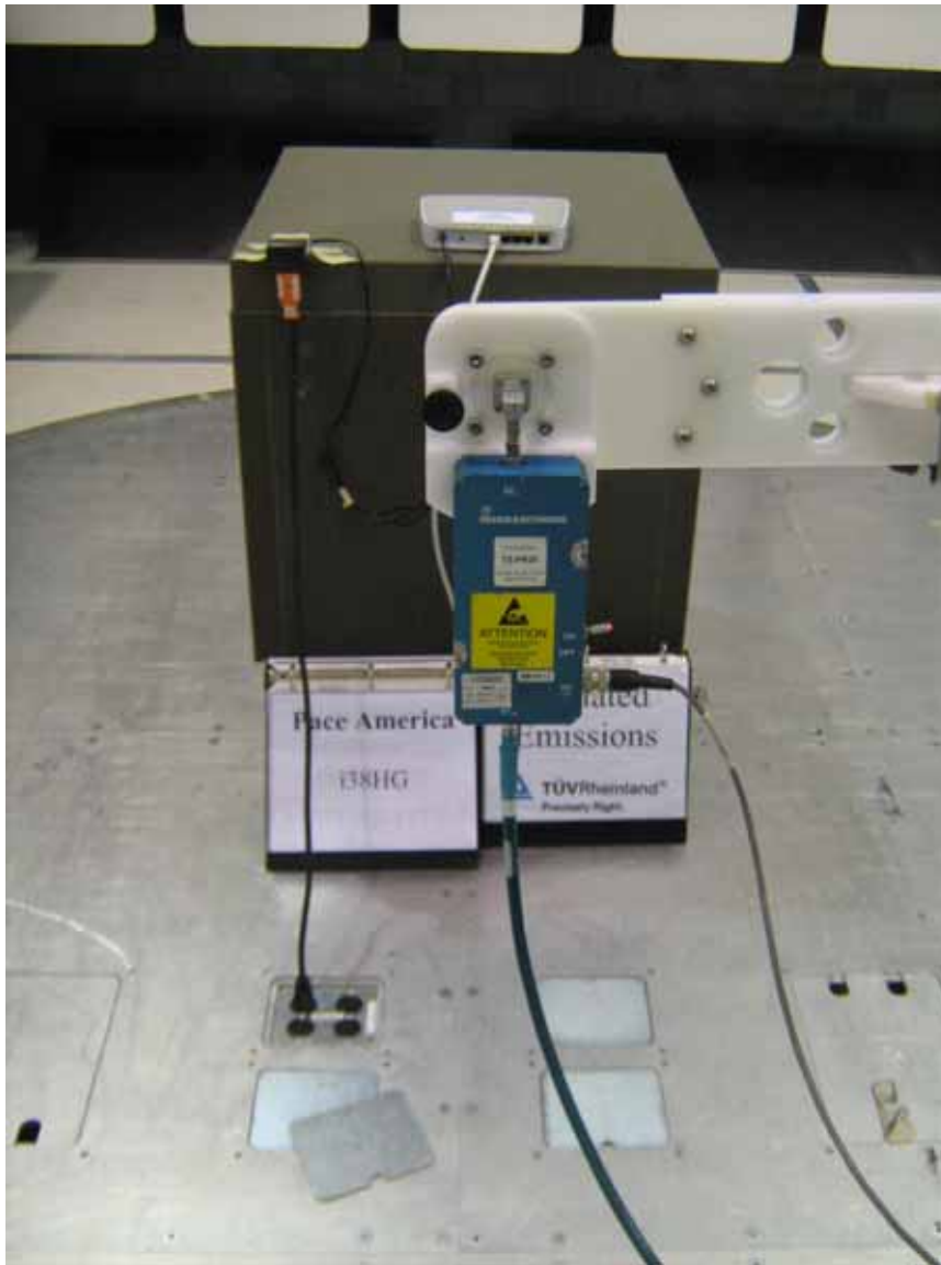
Figure 6: Test Setup for 18 GHz to 26GHz (Rear View) - i38HG on Horizontal Position
