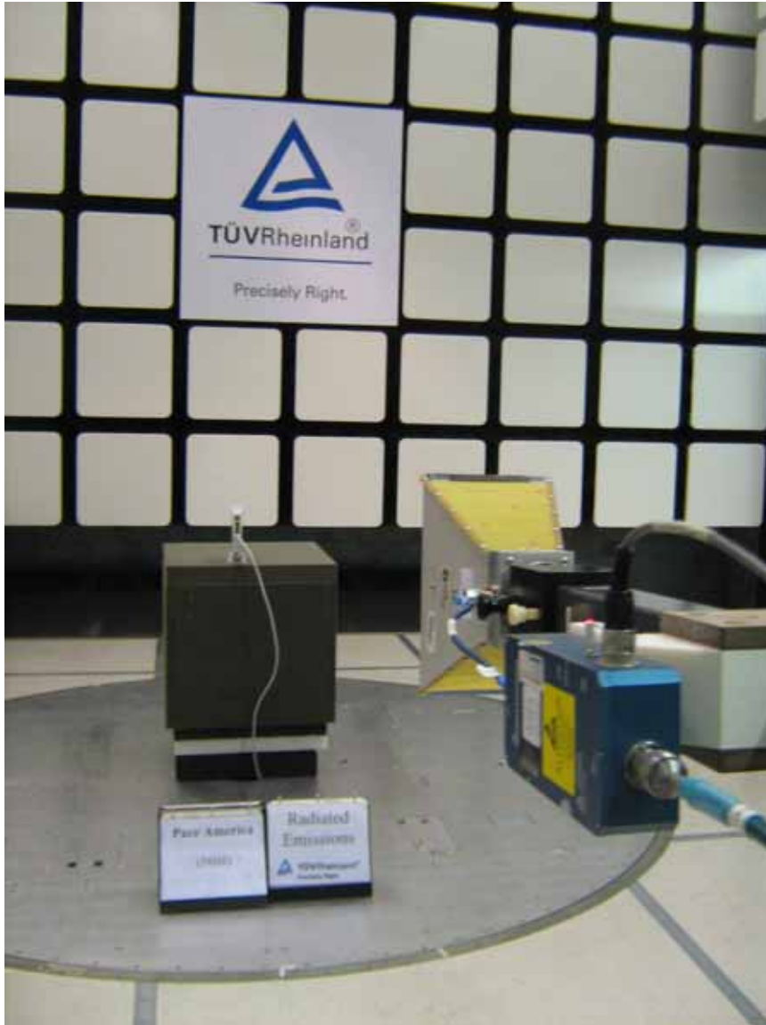
Figure 4: Test Setup for 1GHz to 18GHz (Rear View) – i38HG on Vertical Position
