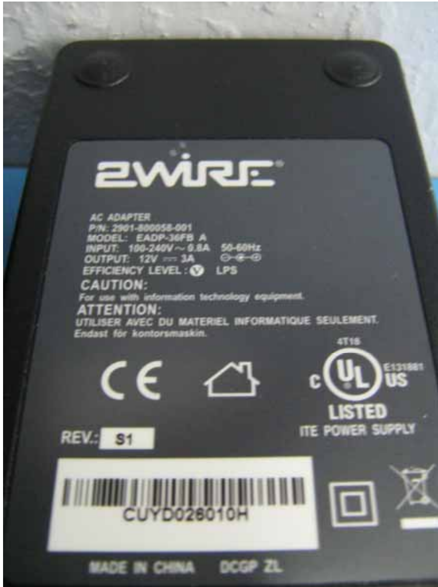
Figure 4: Photo of 5111NV – Power Supply
