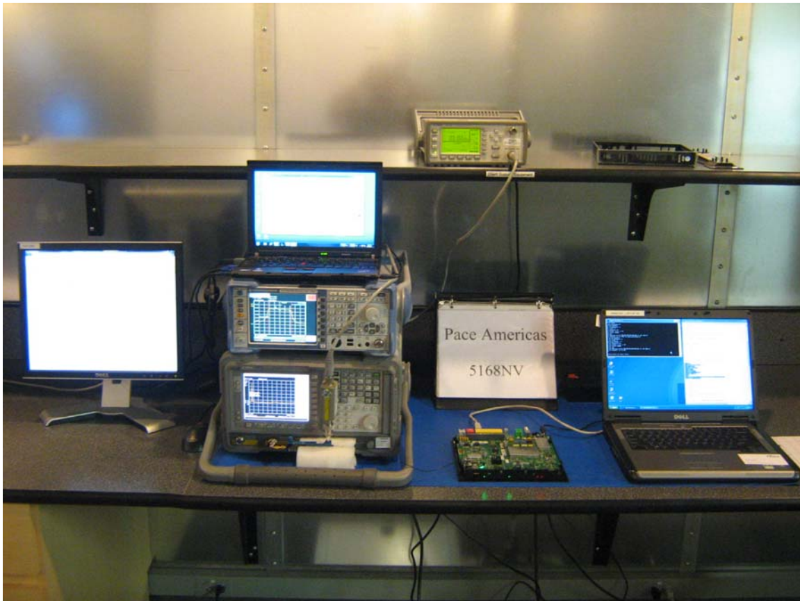
Figure 7: RF Conducted Test Setup
