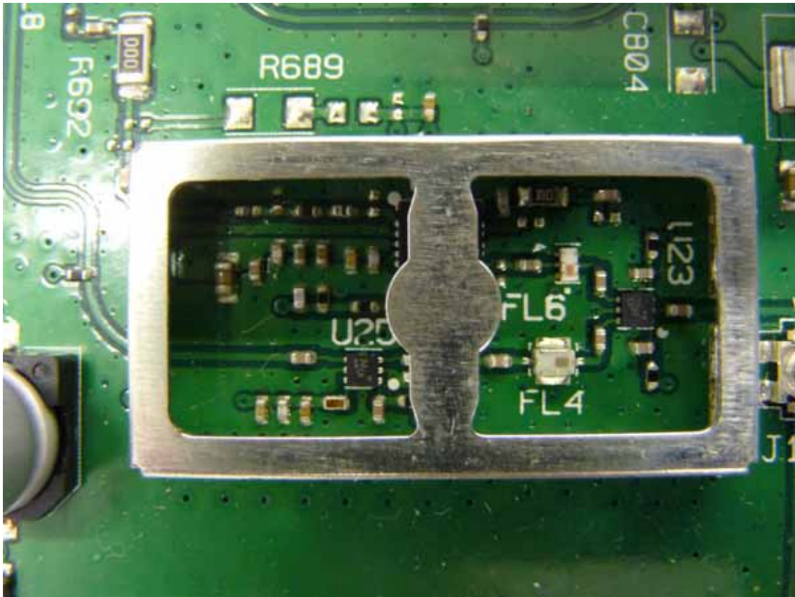
Figure 4: Internal Photo of 5168 – Inside the Chipset RF Can.
