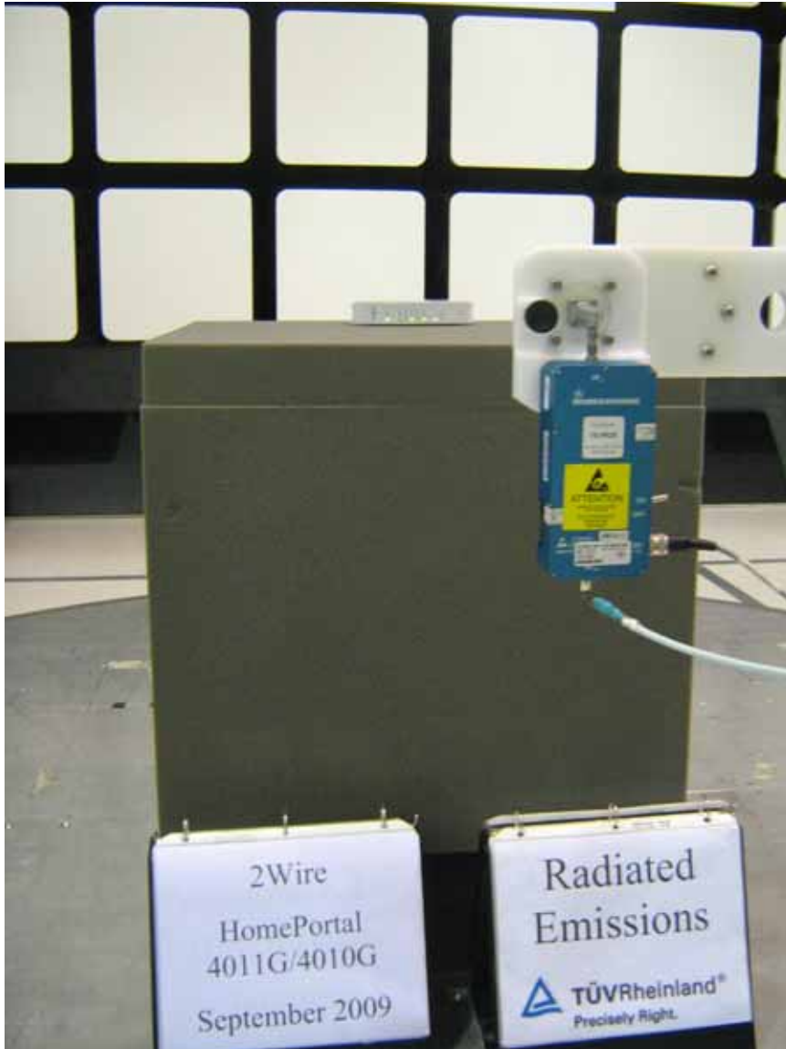
Figure 6: Photo of Test Setup for 4011G/4010G, 18 GHz to 26GHz (Rear View)
