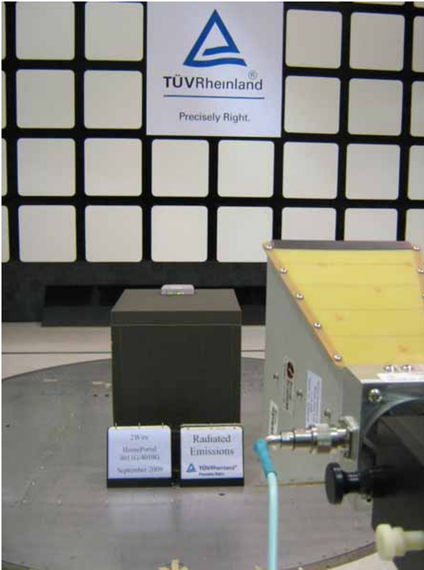
Figure 4: Photo of Test Setup for 4011G/4010G, 1GHz to 18GHz (Rear View)
