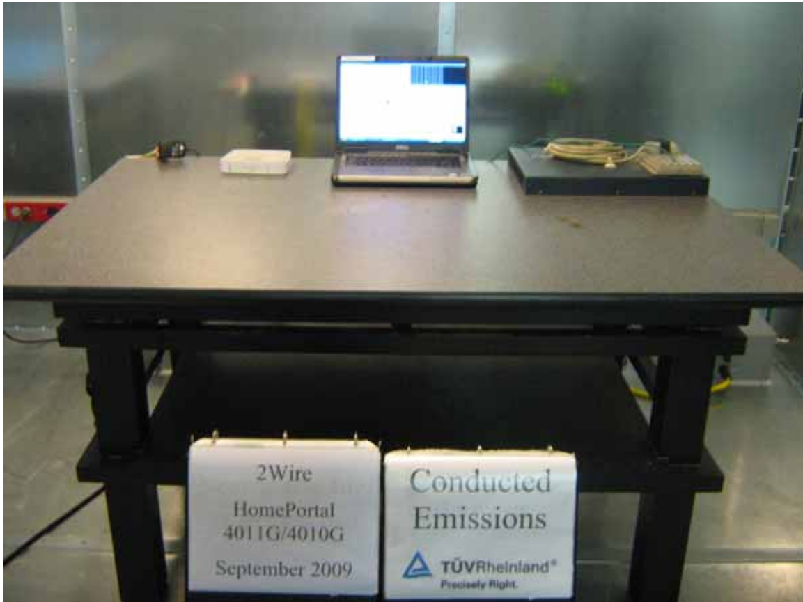
Figure 7: Photo of Test Setup for 4011G/4010G, AC Conducted Emission (Front View)
