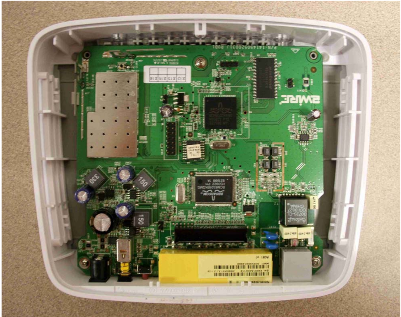
Figure 6: Internal Photo of 4011G/4010G - PCB Board with Shields ON.
