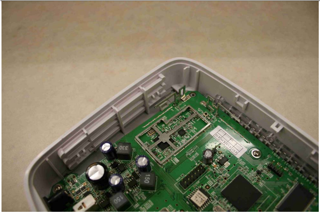
Figure 8: Internal Photo of 4011G/4010G - PCB Board with Shields OFF
