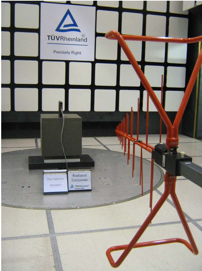
Figure 2: Test Setup for 30 MHz to 1000MHz (Rear View) – 3801HGV on Vertical Position
