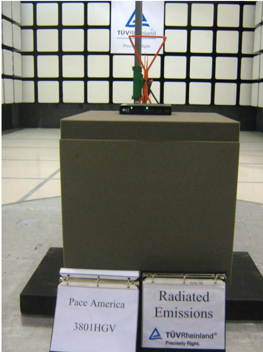
Figure 1: Test Setup for 30 MHz to 1000MHz (Front View) – 3801HGV on Horizontal Position
