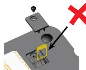
**Never** insert a SIM card frame into the unit without the central SIM card present and securely attached to the outer SIM frame. Doing so will lock the SIM frame inside the unit preventing its removal.
