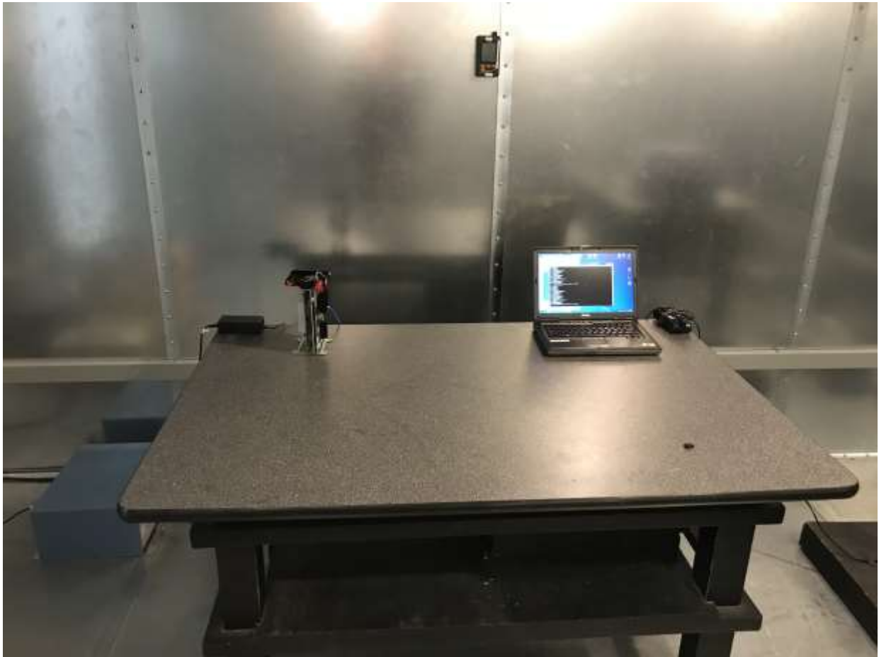
Figure 11: Conducted Emission Test Setup (Front)
