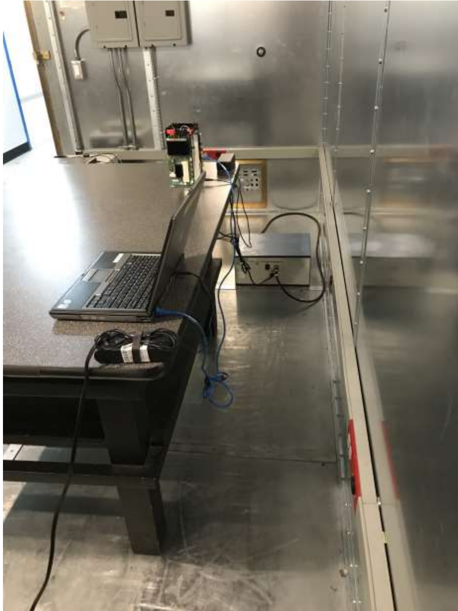
Figure 12: Conducted Emission Test Setup (Side)
