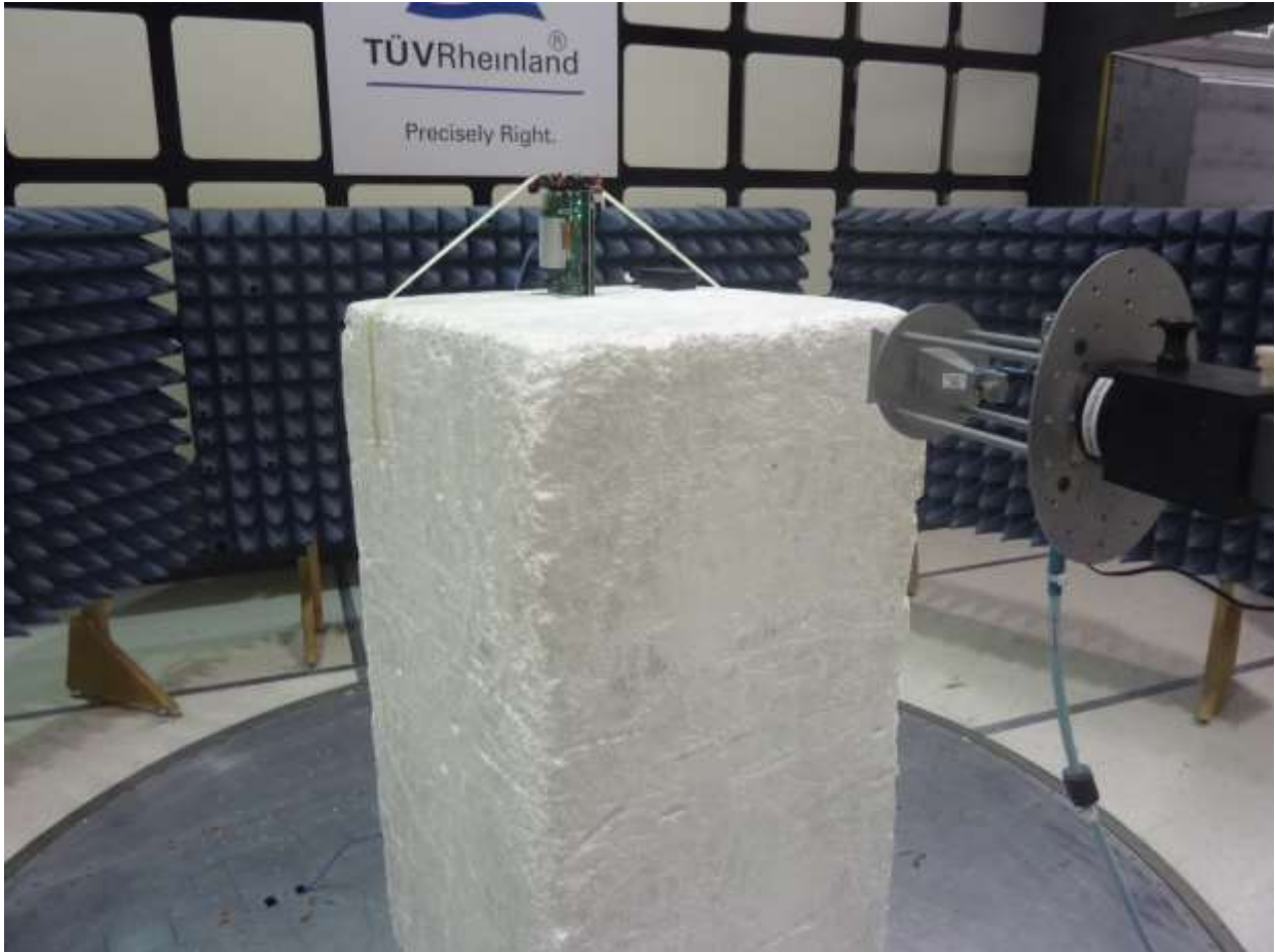
Figure 8: Test Setup for 18 GHz to 26GHz or 40GHz (Rear View)
