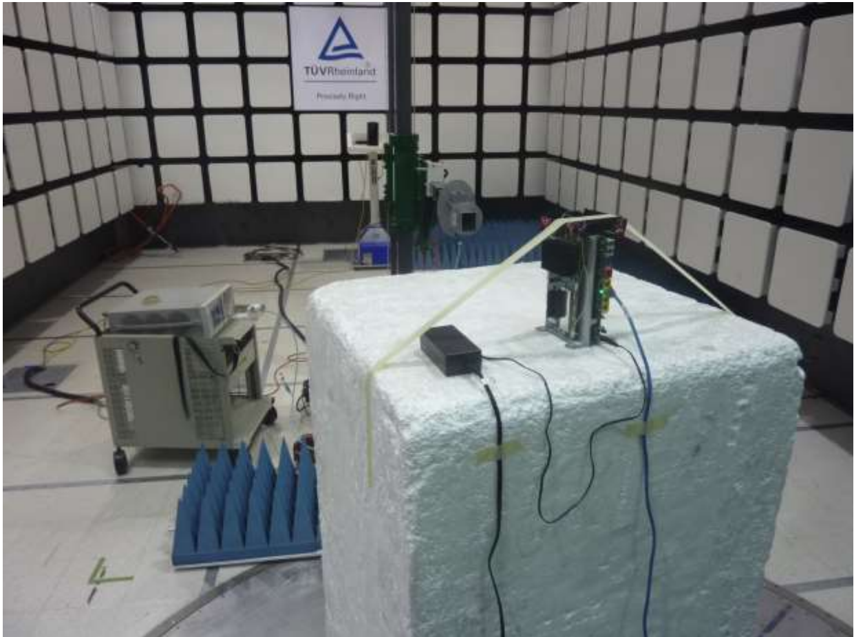
Figure 7: Test Setup for 18 GHz to 26GHz or 40GHz (Front View)
