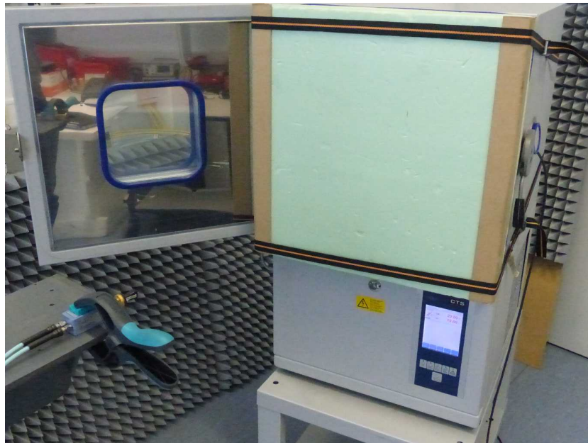
Photo 13: Radiated measurements in climatic chamber
