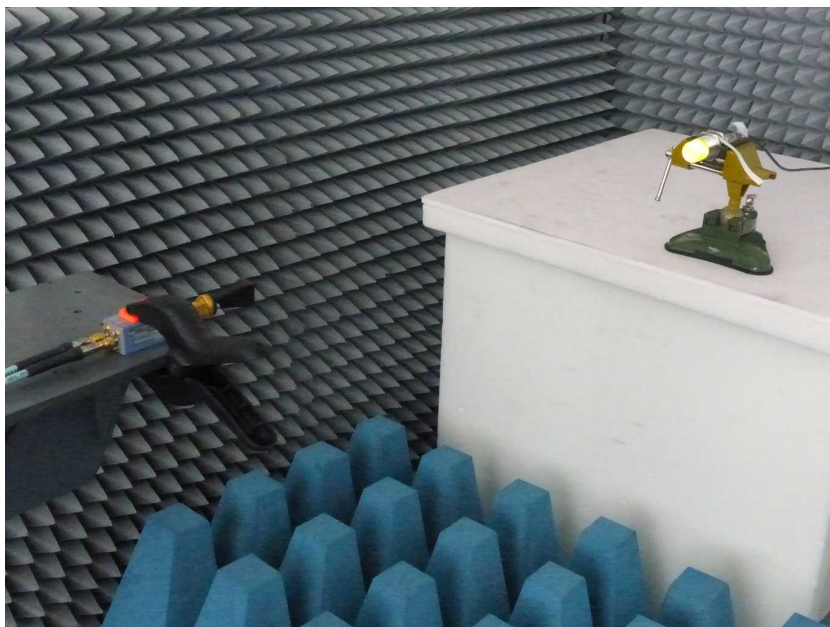
Photo 6: Radiated measurements in test lab
