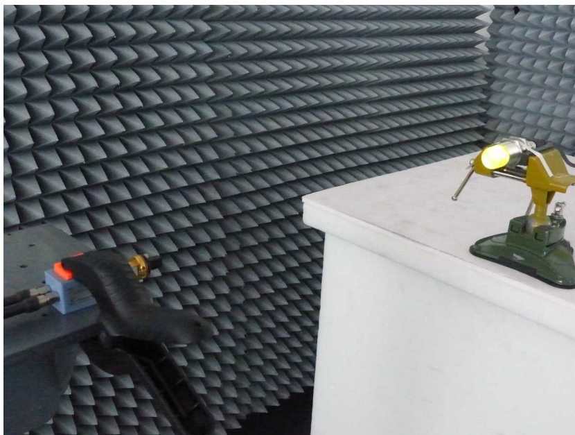
Photo 8: Radiated measurements in test lab
