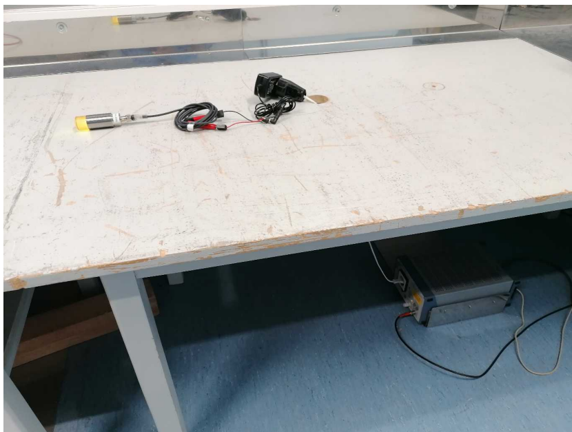
Photo 16: Emissions conducted back onto the AC power line
