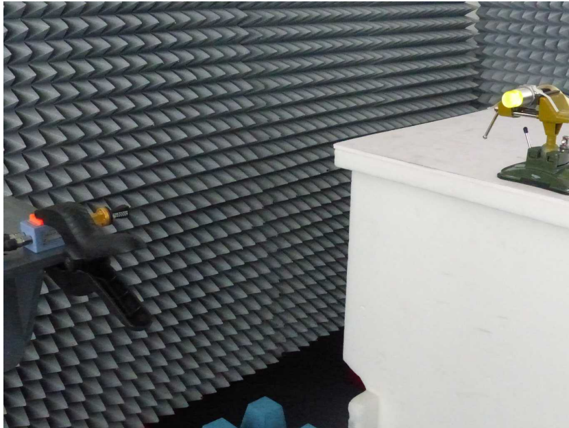
Photo 7: Radiated measurements in test lab
