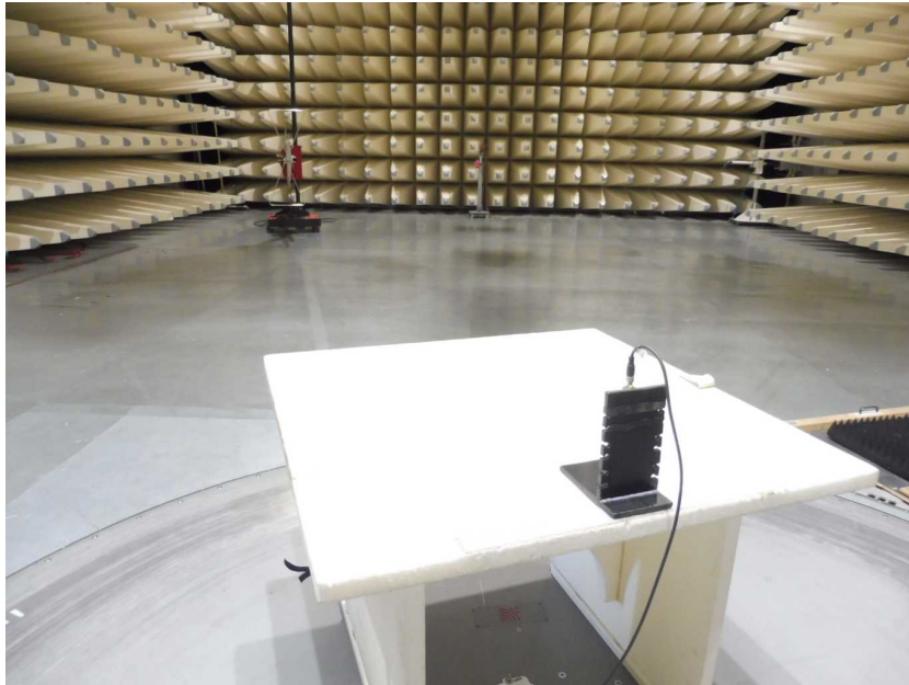
Photo 5: Radiated measurements shielded semi anechoic chamber
