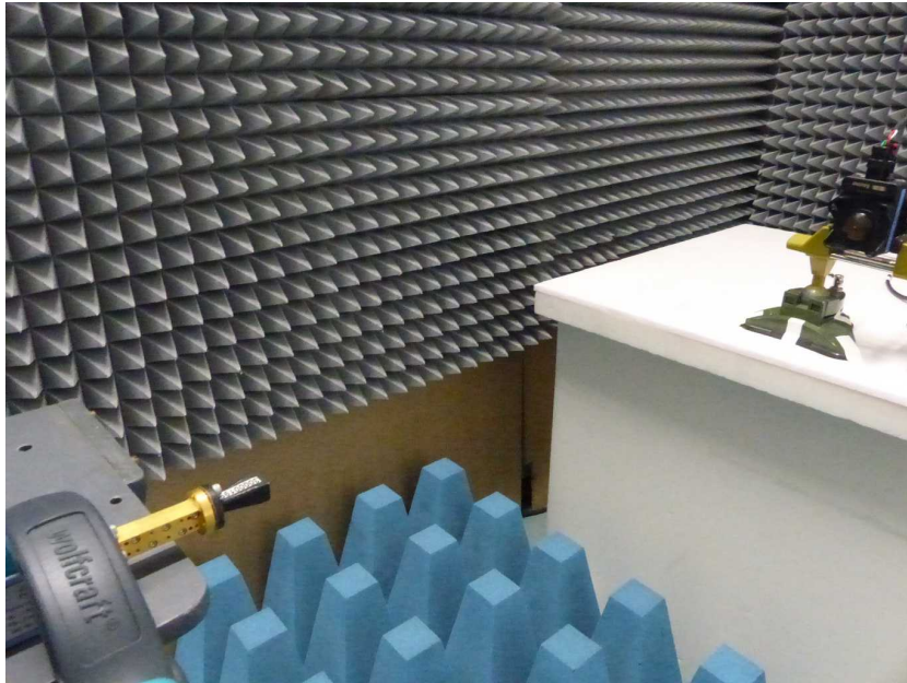
Photo 9: Radiated measurements in test lab
