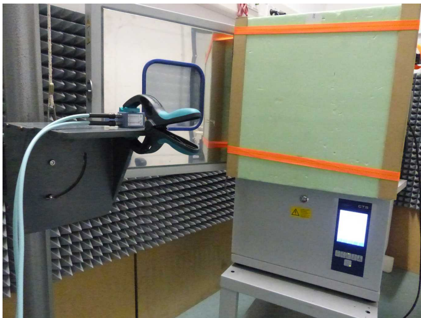
Photo 16: Radiated measurements in climatic chamber
