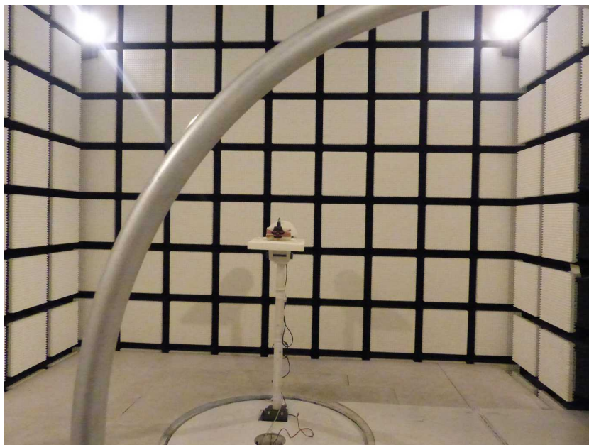
Photo 4: Radiated measurements fully anechoic chamber
