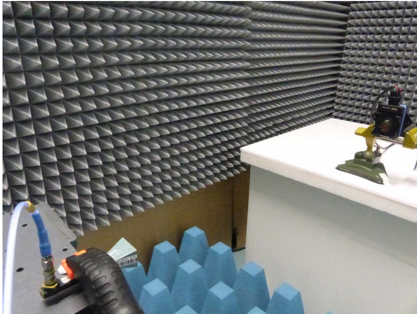
Photo 13: Radiated measurements in test lab
