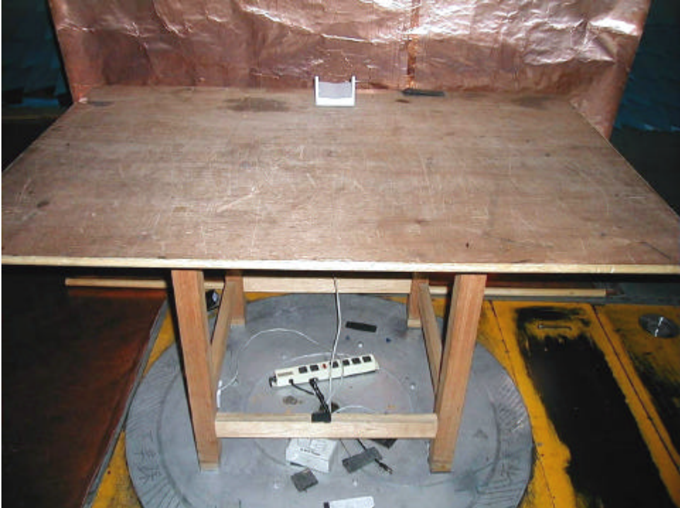
Conducted Emissions Test Placement
