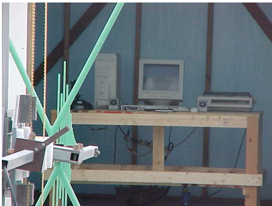
Radiated Emissions (Open Area Test Site), Front of AMERICAN MICROSYSTEMS' M6200
