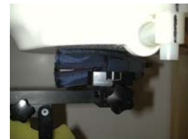
Figure 14.2 Body SAR Test Setup -- w/ Holster --
