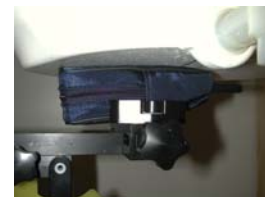
Figure 14.1 Body SAR Test Setup -- w/ Holster --
