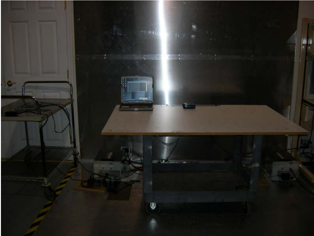
Figure 5.2-3: Conducted Emissions Test Setup
