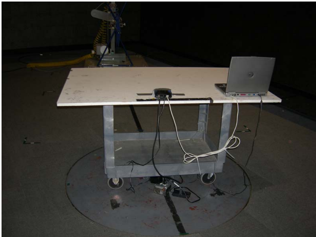
Figure 5.2-2: Radiated Emissions Test Setup - Rear View
