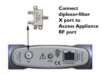
**Note:** Make sure are all connections are secure; if necessary, use a wrench or pliers to lightly tighten the connections.
