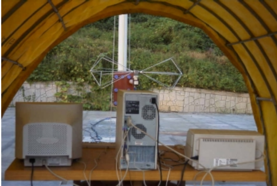
Photograph 1 : Setup for radiated Emissions
