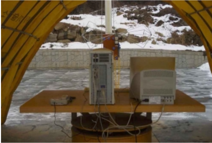
Photograph 1 : Setup for radiated Emissions
