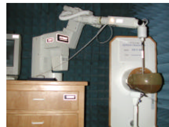
Fig. 1 SAR Test Setup
