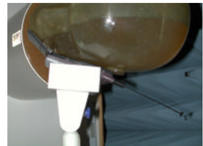
Figure 15. Head SAR Test Setup
