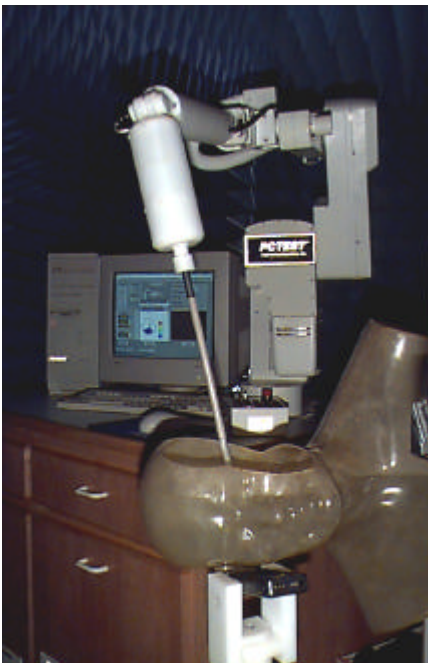
Figure 5. Photograph of the Probe and the Phantom
