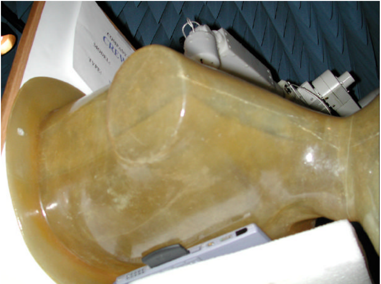
Figure 8. Test Setup of EUT in normal operating position with the source of significant emissions (antenna) 0.5 cm below the phantom.
