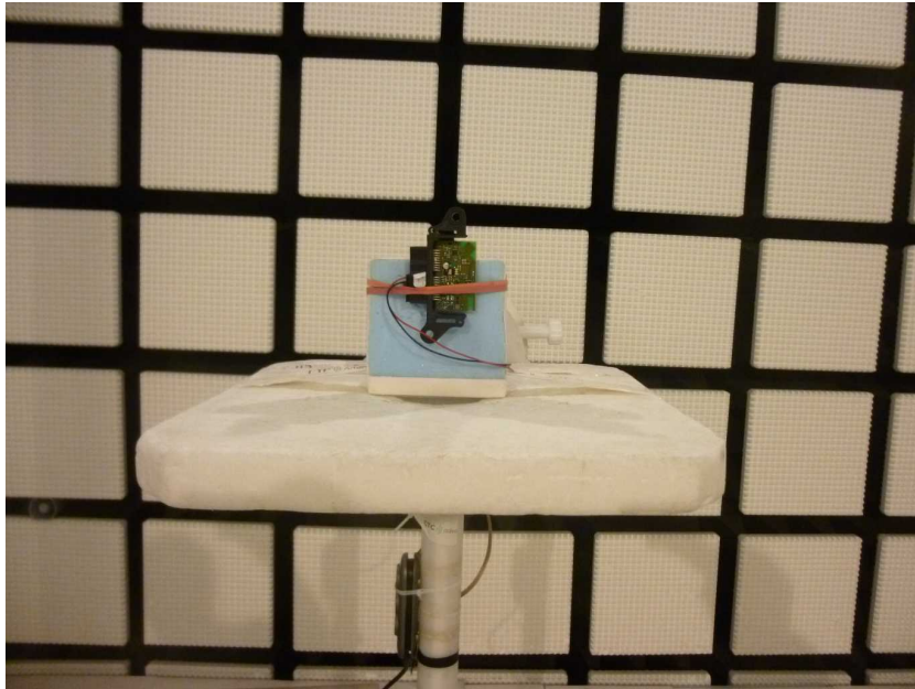
Photo 11: EUT at the anechoic chamber, below 18 GHz test setup
