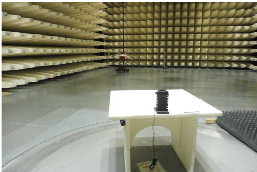
Photo 6: EUT at the semi-anechoic chamber, below 1 GHz test setup
