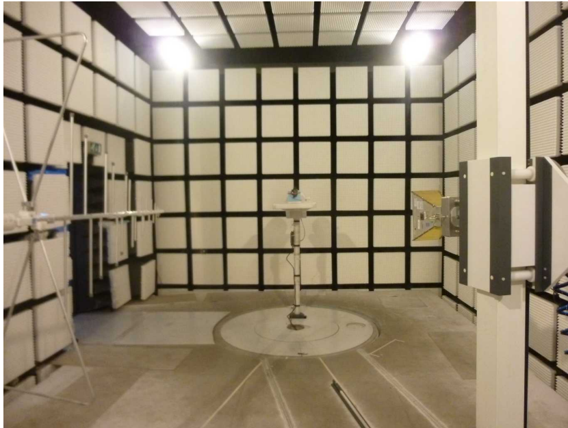
Photo 13: EUT at the anechoic chamber, below 18 GHz test setup
