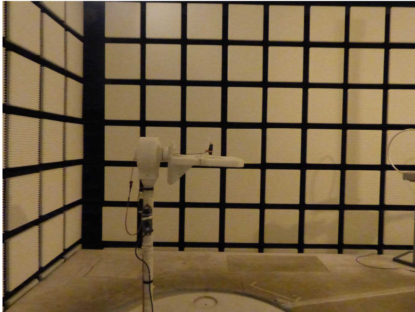
Photo 3: EUT at the fully anechoic chamber
