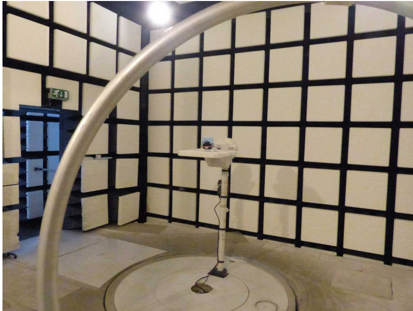
Photo 5: EUT at the fully anechoic chamber
