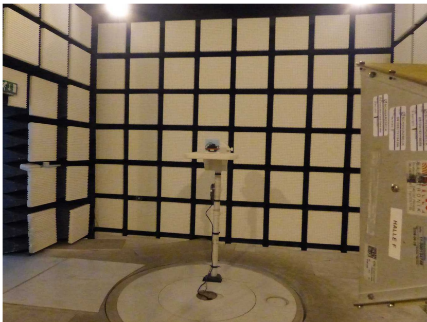
Photo 4: EUT at the fully anechoic chamber
