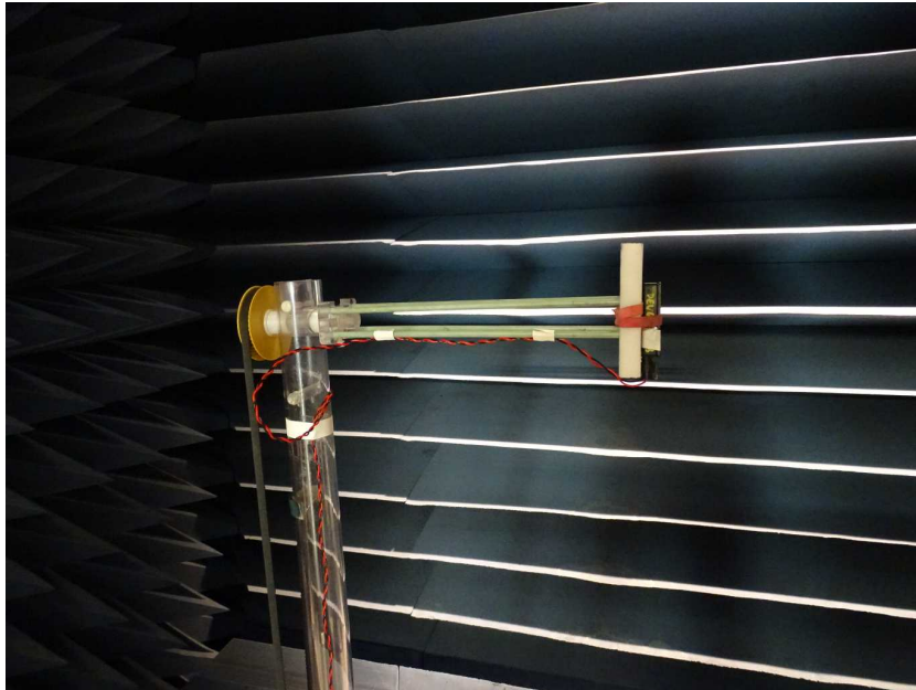
Photo 1: UWB test setup 960 MHz to 10 GHz
