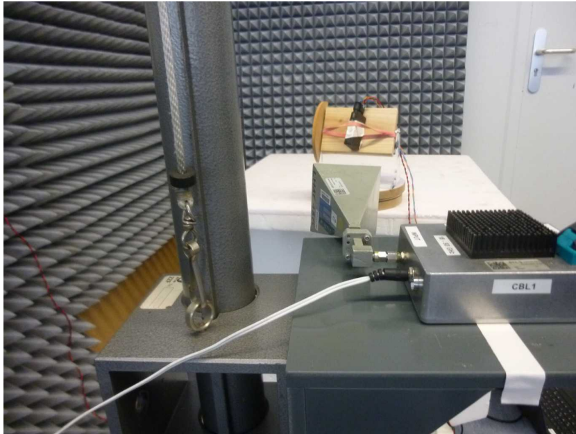
Photo 7UWB 18 GHz to 40 GHz test setup
