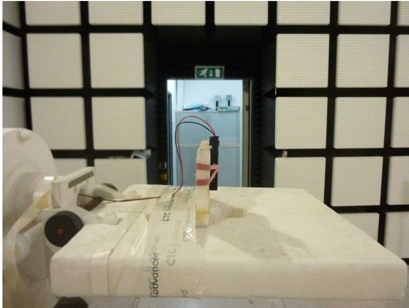
Photo 9: EUT at the anechoic chamber, below 18 GHz test setup
