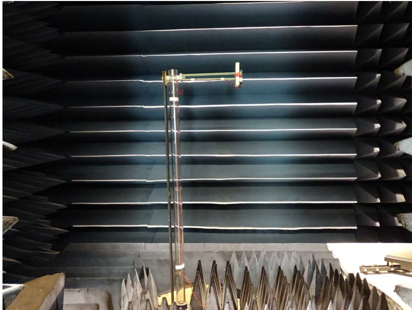
Photo 3: UWB test setup 960 MHz to 10 GHz
