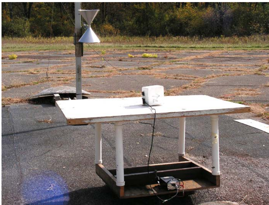
Photograph 6.5. DUT on OATS (one of three axes tested)
