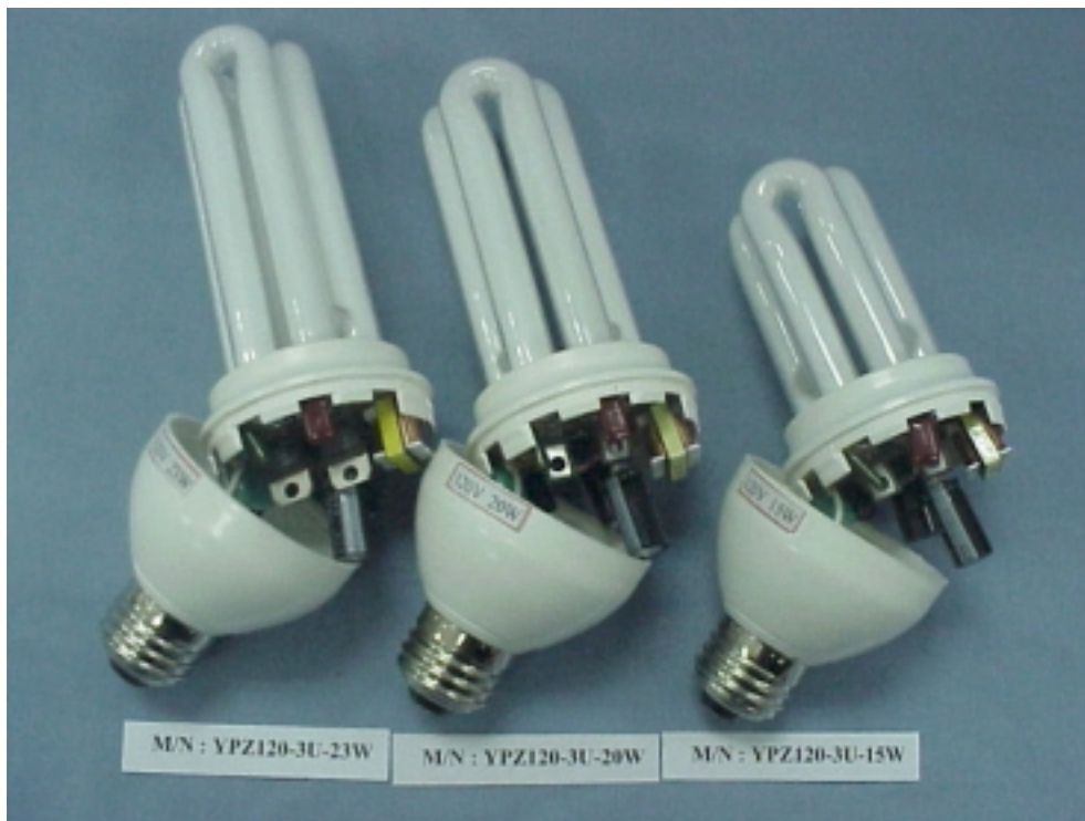
Figure 2 Energy Saving Lamp (M/N: YPZ120-3U Series) MAIN BOARD (COMPONENT SIDE)
