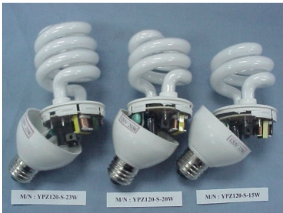
Figure 4 Energy Saving Lamp (M/N: YPZ120-S Series) Cover Removed
