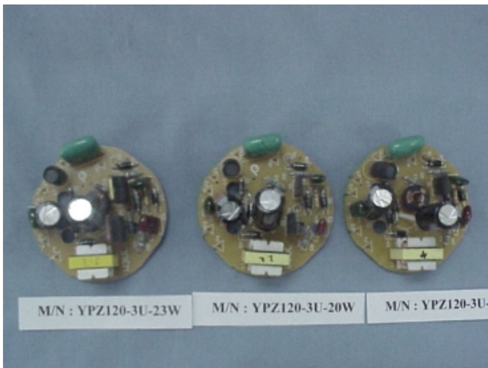
Figure 2 Energy Saving Lamp (M/N: YPZ120-3U Series) MAIN BOARD (COMPONENT SIDE)
