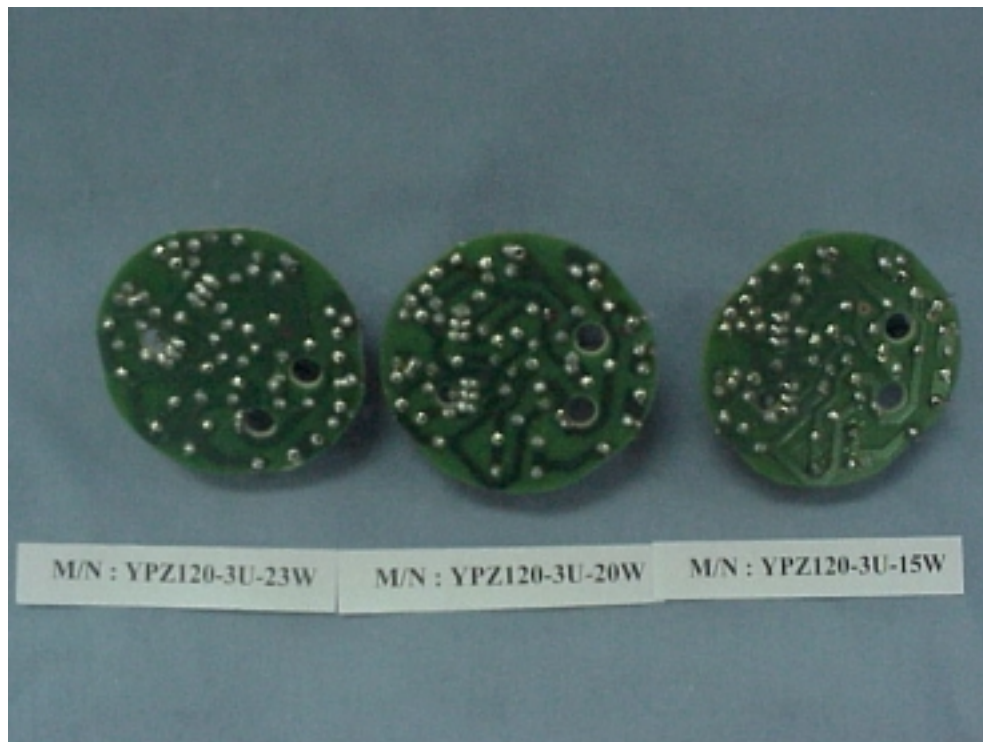
Figure 4 Energy Saving Lamp (M/N: YPZ120-S Series) Cover Removed
