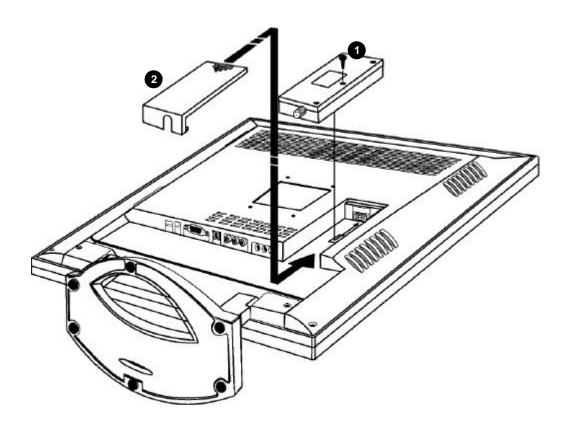
Note :1) For your convenience, the TV Tuner module has been installed at the factory. The illustration is shown for your reference only.
