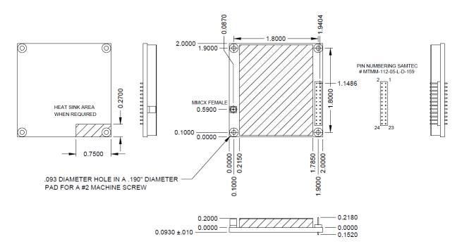
The four mounting holes have a 0.093" diameter finished opening 0.100" from the edges designed for a #2-56 screw. The clearance height of the radio is 0.210" shield height, .103" PCB height, 0.070" back side height. (The connectors are on the side with the shield.)
