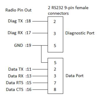
Depending upon configuration, before connecting to a computer, each serial port may need to pass through a 3.3V TTL to RS232 converter such as this SerialComm TTL-232-33P. The radio is either manufactured for a high speed 3.3V interface or for a conventional speed RS-232 interface.
