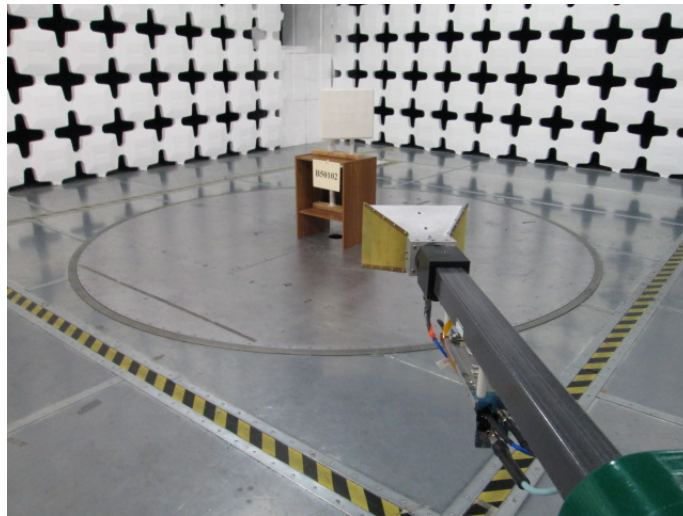
Test Setup – Radiated Emissions (above 1 GHz)
