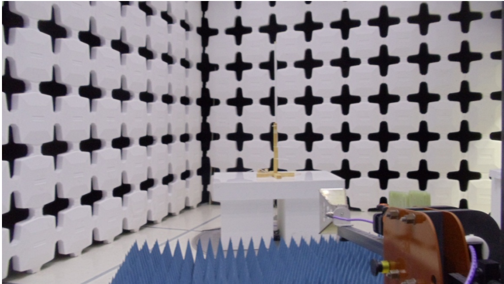
Test Setup for Radiated Emissions, 1GHz to 10GHz – Horizontal Polarization – Laird Antenna
