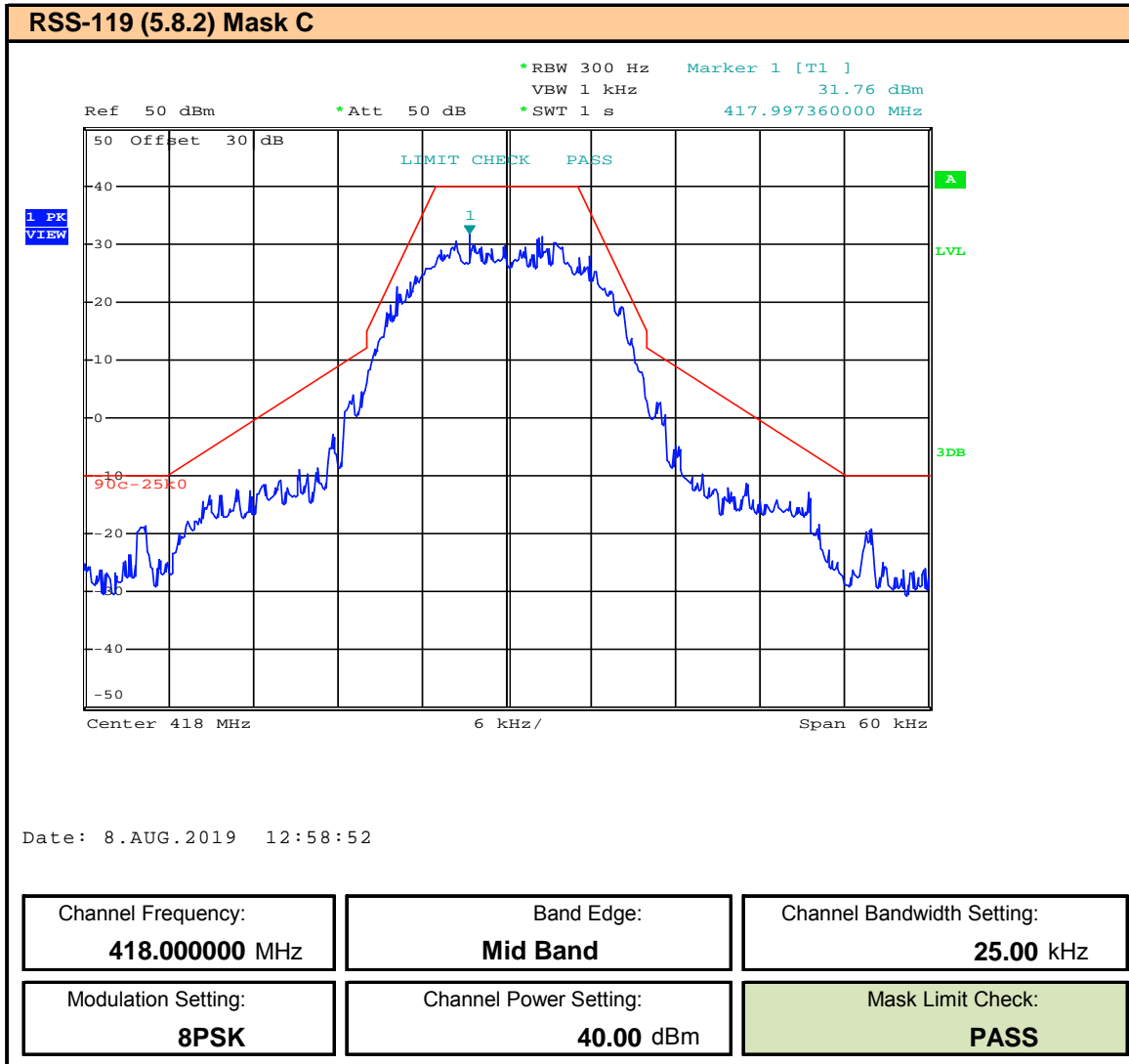
Plot 9.53 – Band Edge and Emissions Mask – 25kHz BW – 8PSK – 418MHz, ISED
