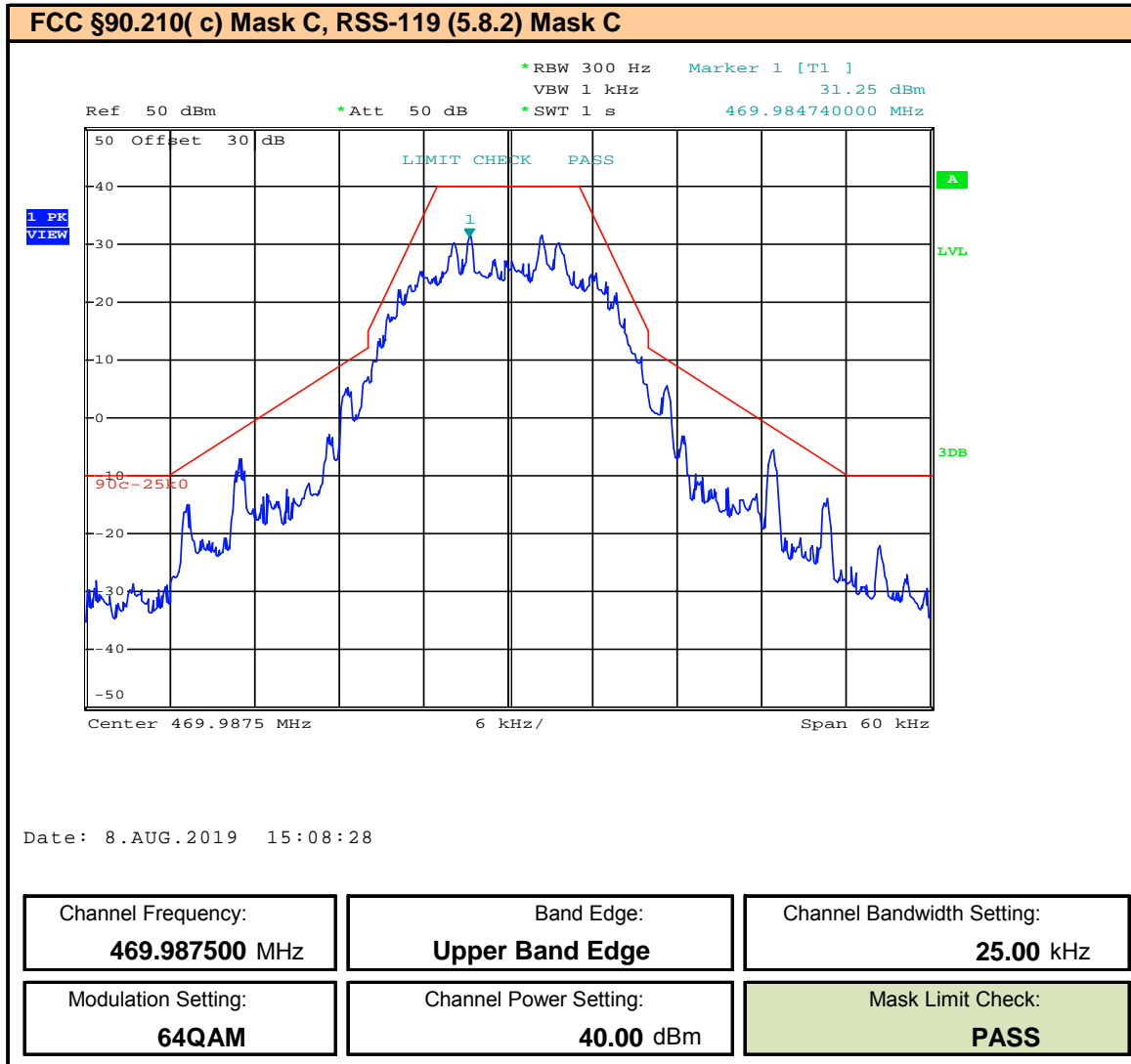
Plot 9.81 – Band Edge and Emissions Mask – 25kHz BW – 64QAM – 469.9875MHz
