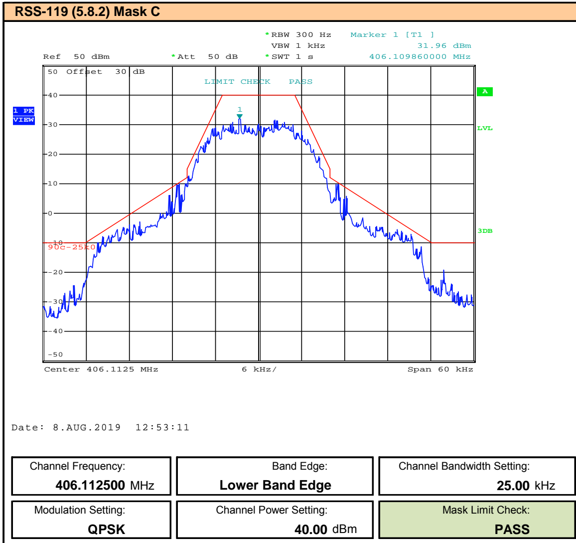
Plot 9.58 – Band Edge and Emissions Mask – 25kHz BW – QPSK – 406.1125MHz, ISED
