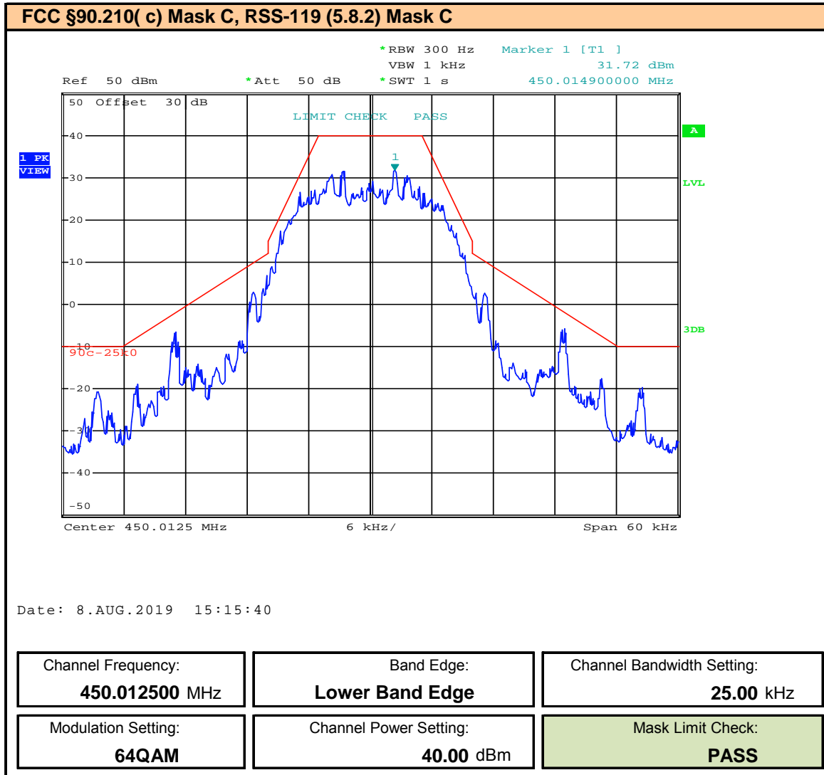
Plot 9.79 – Band Edge and Emissions Mask – 25kHz BW – 64QAM – 450.0125MHz
