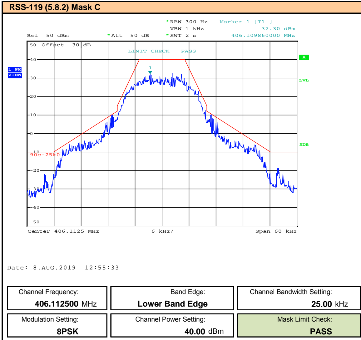
Plot 9.52 – Band Edge and Emissions Mask – 25kHz BW – 8PSK – 406.1125MHz, ISED
