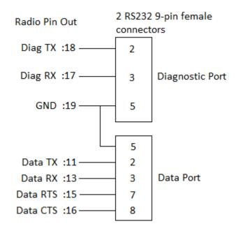
Depending upon configuration, before connecting to a computer, each serial port may need to pass through a 3.3V TTL to RS232 converter such as this SerialComm TTL-232-33P. The radio is either manufactured for a high speed 3.3V interface or for a conventional speed RS-232 interface.
