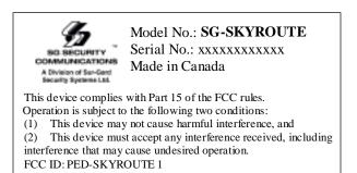
The FCC Label (4.00" x 1.00") is placed on the back of the metal bracket that holds the PCB and the radio modem. Please see attached drawing.
