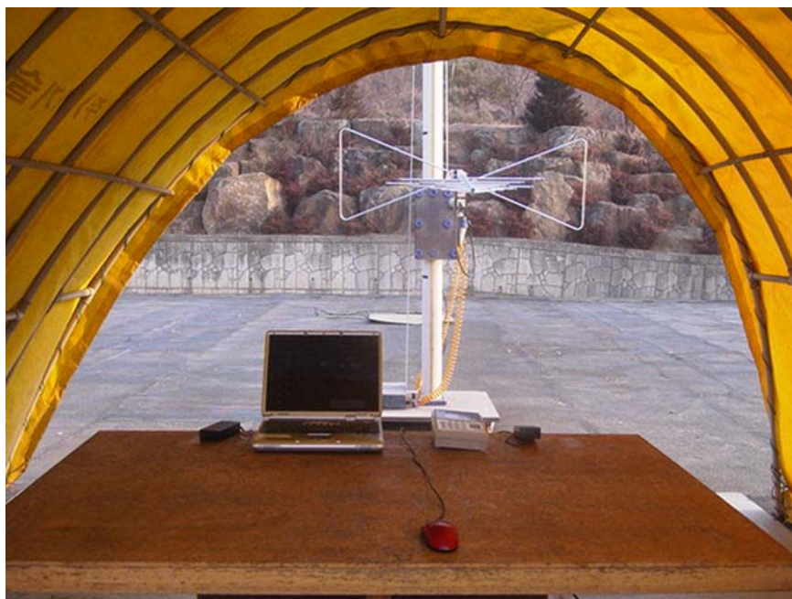
Photograph 1 : Setup for radiated Emissions
