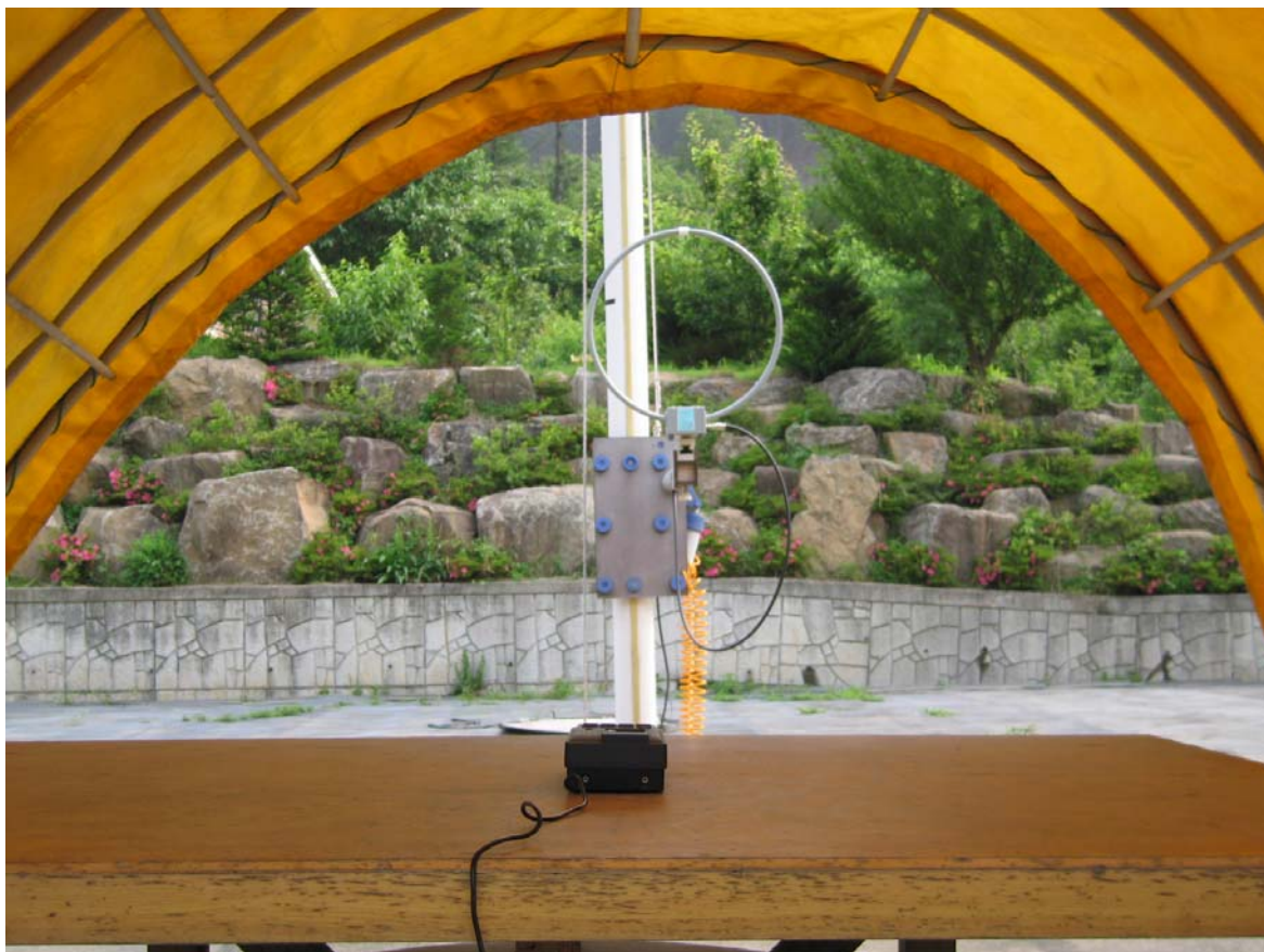
Photograph 3 : Setup for Field strength
