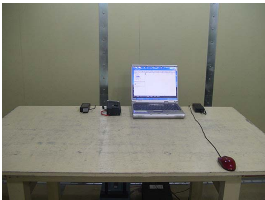
Photograph 2 : Setup for Conducted Emissions
