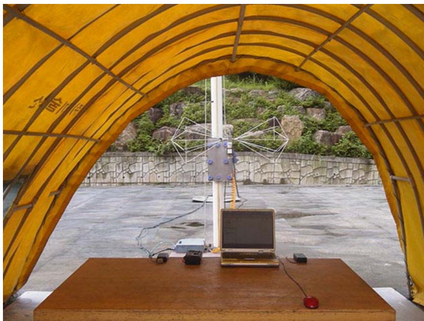
Photograph 1 : Setup for radiated Emissions
