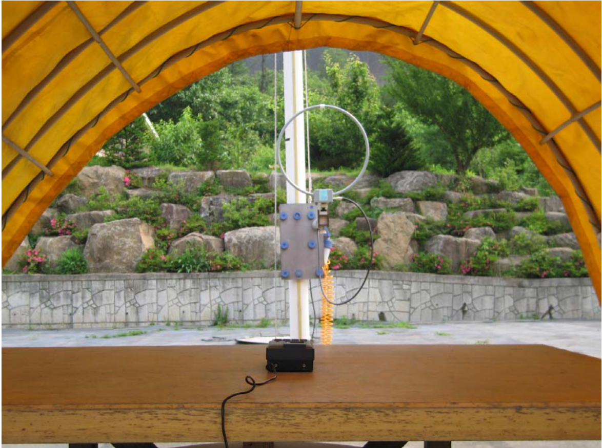
Photograph 3 : Setup for Field strength
