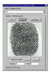
4)If you click <Start> after selecting check box "Continuous Capture", then fingerprint image appears continuously. At this time, information about the action state of the device appears below.
