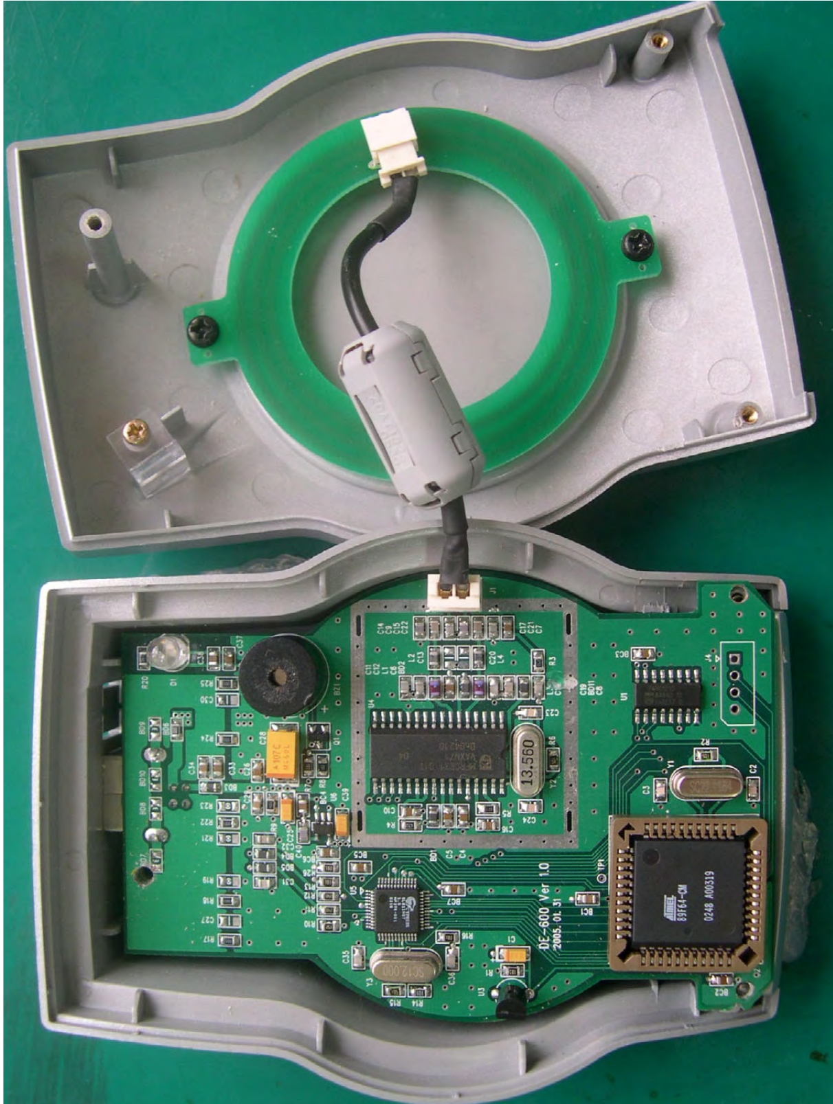
<Photograph 12: RFID Card Reader cover removed>
