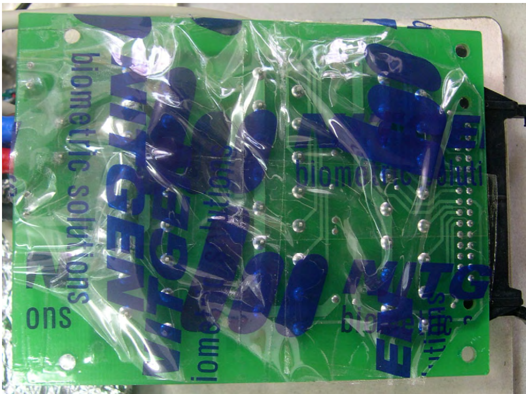
<Photograph 3: I/O board - Rear View>
