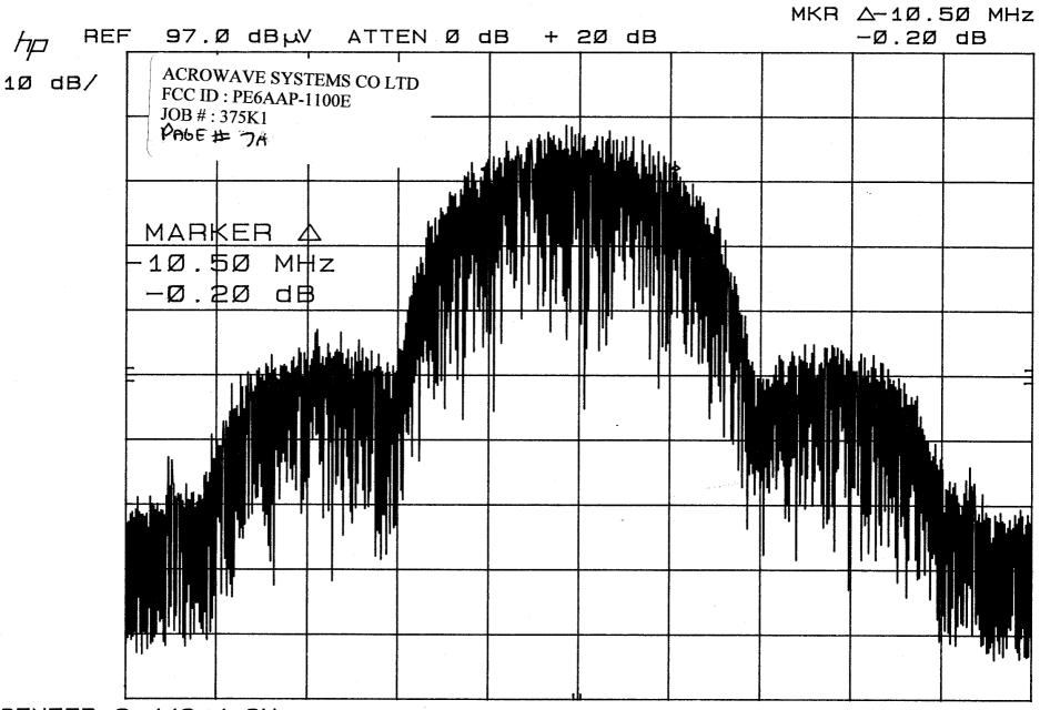
CENTER 2.442 4 GHz RES BW 100 kHz (i) VBW 300 kHz SPAN 5Ø.Ø MHz SWP 37.5 msec
