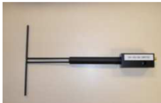
Figure 1 – Satimo COMOSAR Validation Dipole
