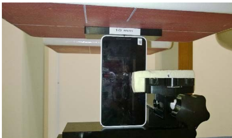
Photo of the device positioned for WR mode measurement – bottom edge facing phantom. The spacer was removed before the start of the measurements.
