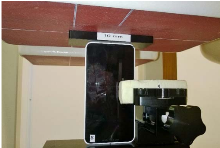
Photo of the device positioned for WR mode measurement – top edge facing phantom. The spacer was removed before the start of the measurements.
