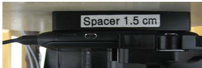
Photo of the device positioned for Body SAR measurement. The spacer was removed for the tests.
