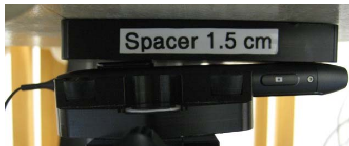
Photo of the device positioned for Body SAR measurement. The spacer was removed for the tests.
