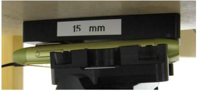
Photo of the device positioned for Body SAR measurement.
